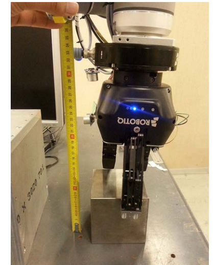
Distance measurement from the S_S1 sensor and collision detection
