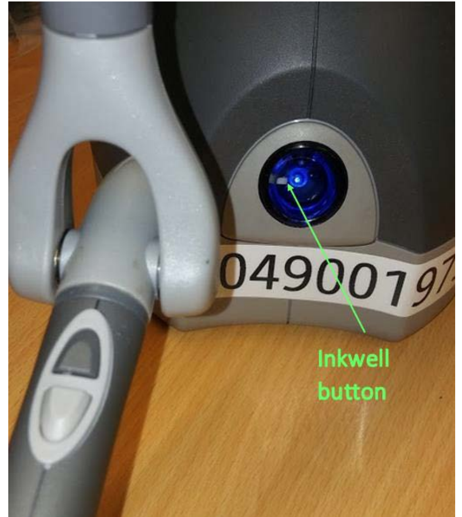
Inkwell, white and grey buttons of Geomagic Touch device
